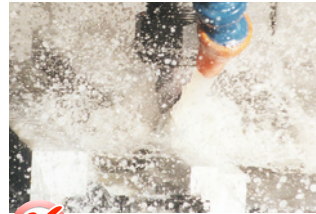
Machining with flood coolant
