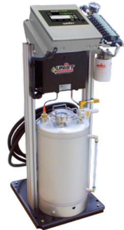
The auto refill fluid supply system incorporates a 10 gallon [38 liter] ASME rated stainless steel pressure tank with 0-60 psi [0-4 bar] precision regulator and integral high and low level switches. The system also includes PLC controls and an electric pump to automatically refill the tank, which eliminates down time. This system provides superior performance when drawing fluid from a tote or drum.
