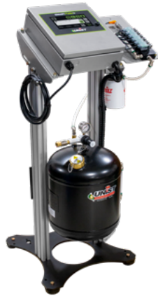
The 6 gallon [22 liter] ASME rated pressure tank comes equipped with a 0-100 psi [0-7 bar] regulator, low level switch and sight gauge.
