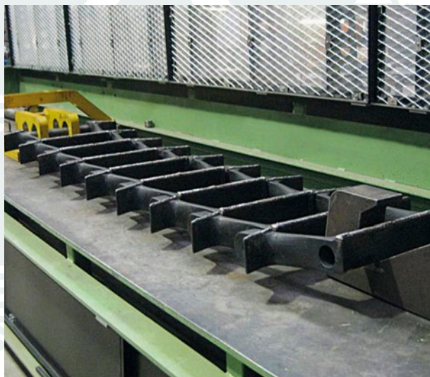
Proof testing of cast chains is carried out as a matter of routine to ensure total product integrity.
